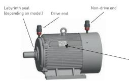
Lubrication points are located on the **drive** and **non-drive end of electric motors**. When relubricating, you must ensure that **excess grease is discharged** through the discharge openings, grease relief ports or grease traps. Bearings will overheat if grease cannot escape and / or if grease traps are filled up with used grease.
